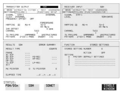
**TRANSMIT** Allows control of the settings associated with the generated signal.
